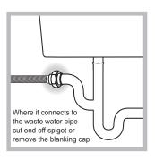
The drain hose may be connected to an under-sink trap. Before connecting the drain hose from the machine ensure that any blanks or removable ends have been taken off the spigot.
